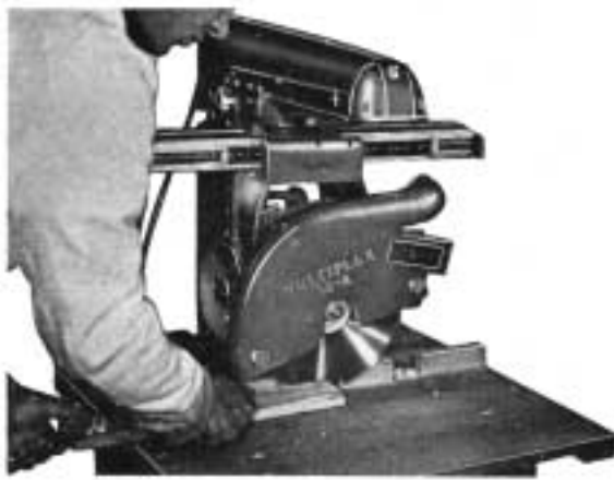
Fig. 2. No. 608009 — Because the adjustment is so important it is recommended that a test block be used to obtain such adjustment. Test block is first cut as shown in this illustration.
