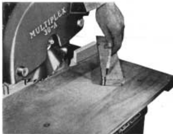
Fig. 4. No. 60810 — This illustration shows typical cuts made on the test block. Note that the cut made in Figure 3 (indicated by pencil) is outside the cut made in Figure 2 and therefore satisfies conditions set forth in Figure 1.
